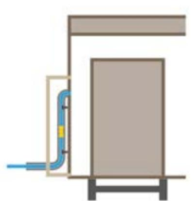
Run the pipework directly to the site cabin with a double check valve on the main feed.
