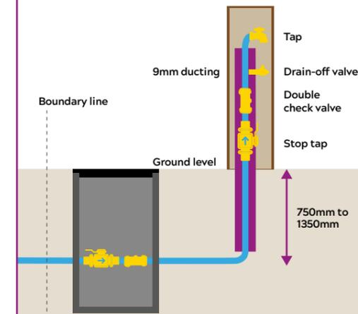
Your pipework fittings and tap must be securely attached to a fixed post or structure. For additional protection we recommend housing in a waterproof lockable box to prevent unwanted third party use.
