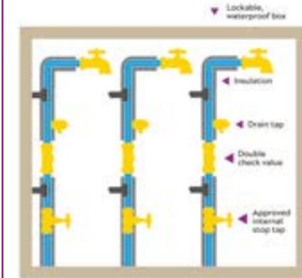
Where multiple standpipes are fitted, each must have a separate stop valve to isolate the tap.
