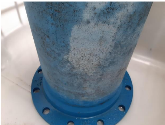
Figure 5 & 6 flanged ends with 100mm of QD8 coating up the barrel from bottom of pipe standing on the tank floors
