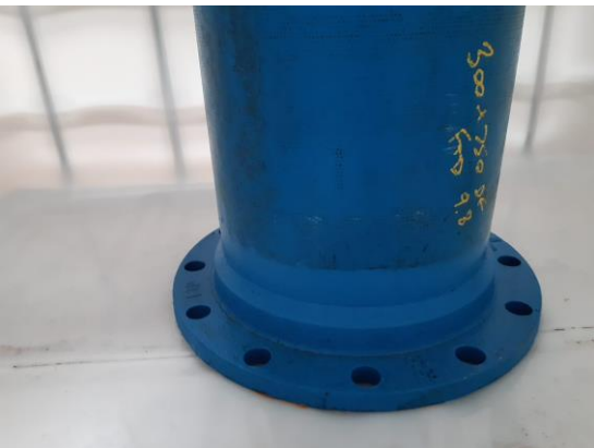
Figure 5 & 6 flanged ends with 100mm of QD8 coating up the barrel from bottom of pipe standing on the tank floors
