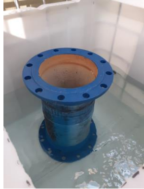
Figure 1 & 2 double flanged ended pipes with 100mm of QD8 coating up the barrel from bottom of pipe standing on the tank floors
